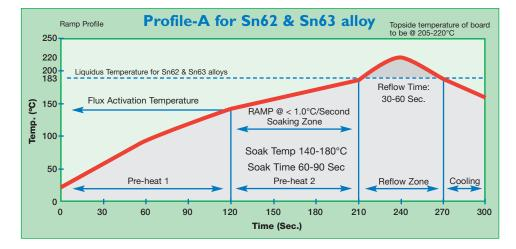
A profile utilizing a soak of up to two minutes at 155°C may help to minimize voiding in BGA assembles. This will allow more time for solvent components of the solder paste to outgas prior to reflow.
