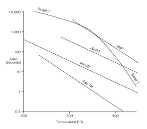
Savbit solder has been used by leading electronics manufacturers throughout the world for over forty years. Savbit was originally used to increase the life of copper soldering iron bits. Soldering speed and efficiency are increased by keeping the iron in good condition. Ironplated bits having a longer life than plain copper tips are now commonly used but they also fail eventually (usually by cracking of the plating) and then erode rapidly unless Savbit solder is used.
